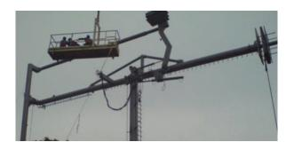
**Fabrication and Trial Fit Loading Arm**
